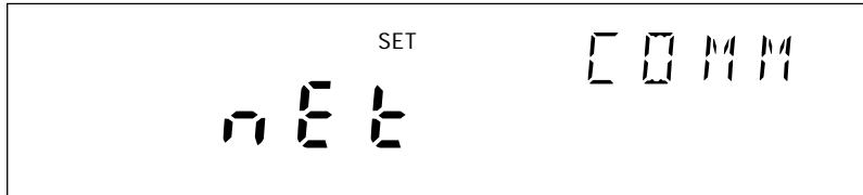
Communications display for setting the network type
